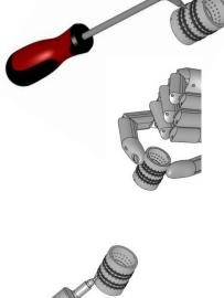
Lubricate O-rings on main sleeve assembly. Spread lubricant evenly across the O-rings. Clear any holes blocked with lubricant.
