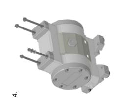
Use 3 mm Allen Wrench to remove outlet manifold.
