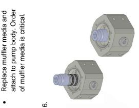
Press Main Shaft Assembly into Body. Take care that the O-rings do not displace themselves from the main sleeve assembly.
