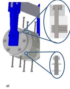
Thread tie bolts onto head retaining rings, align head side 1, body, head side 2, and retaining Washer order is critical. DO NOT TIGHTEN. ring 2 onto tie bolts and clamp together. Apply antiseize lubricant to each tie bolt
