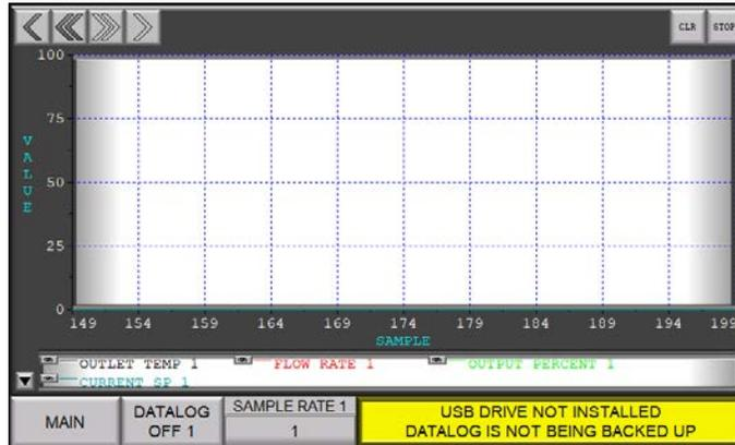
**Figure 16: Trend Graph Display, with message about USB drive not-installed**
