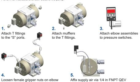
Loosen female gripper nuts on elbow assemblies and T fittings. Insert tubing and hand-tighten gripper nuts.
